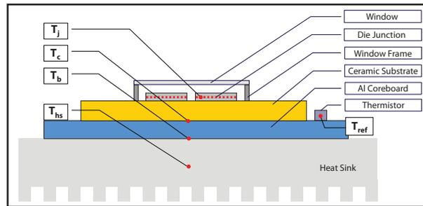
Figure 1: Cross-Section of a Multi-Chip Module
