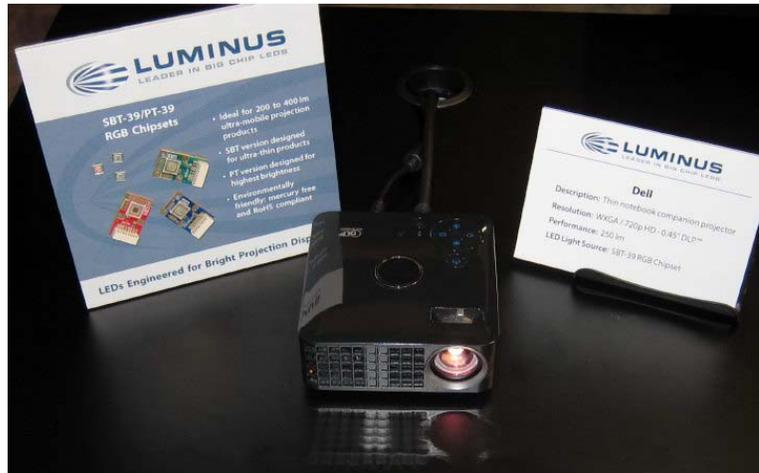
WVGA DLP imager and produced 50 lumens. The photo shows this Dell projector and a Luminus placard that compares the SBT-39 surface mount chipset compared to the conventional PT-39 chipset. The small size of the surface mount version is clearly visible compared to the regular version. —*Matthew Brennesholtz*
